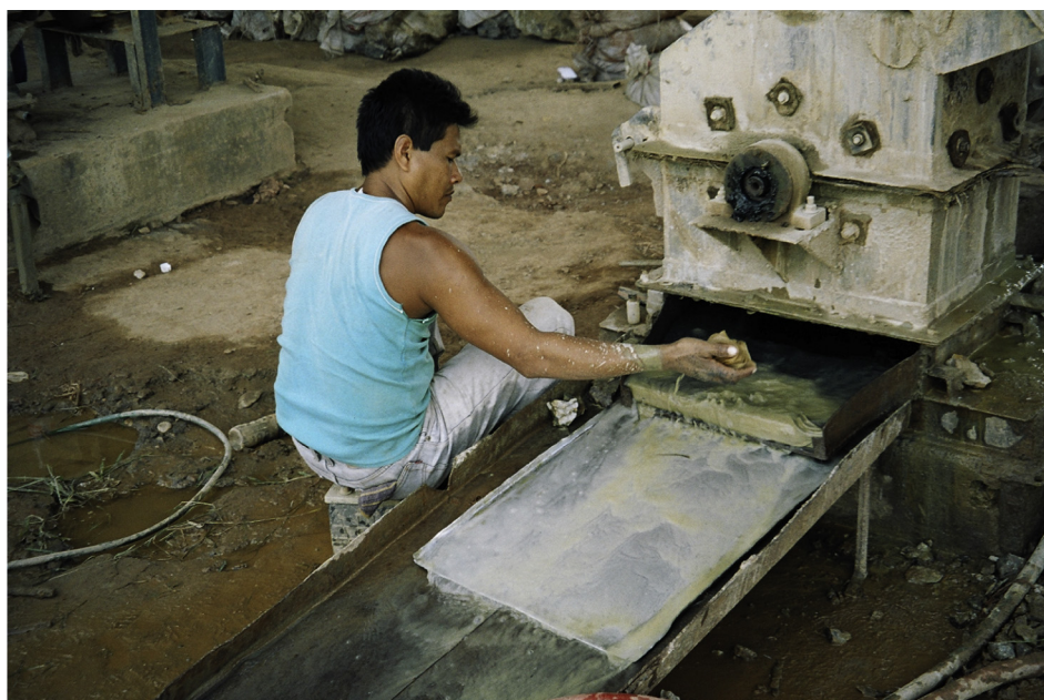
Fig. 1. Venezuelan miner amalgamating the whole ore using a hammer mill and a copper-amalgamating plate.
