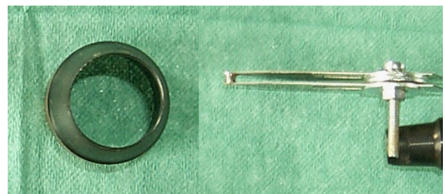
Fig. 1 – Punch used to cut a cylindrical shaped specimen (left) and home-made double-blade scalpel used to prepare from the cylindrical specimen a sample of homogeneous thickness (right).
