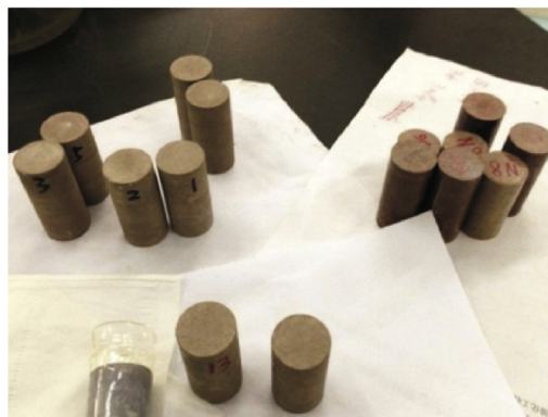
Fig. 1. Devices and cores for the stress sensitivity experiment.
