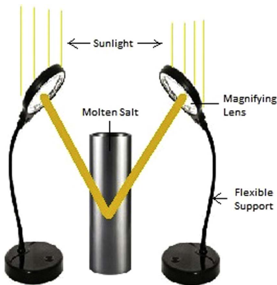
Fig. 1. Heating mechanism for molten salt, where magnifying lenses are used to focus sunlight at one point to heat the molten salt [3–7,11,17,18].
