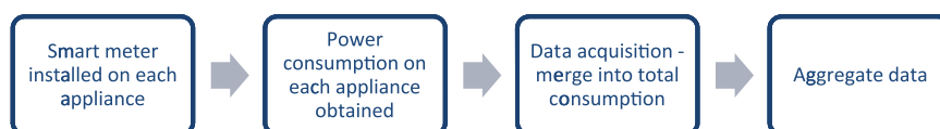
Fig. 1. Intrusive Load Monitoring process using smart meter by measuring individual appliance power consumption.
