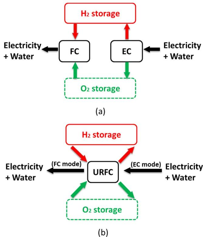
Fig. 1. Comparison between RFC and URFC: (a) RFC; (b) URFC.
