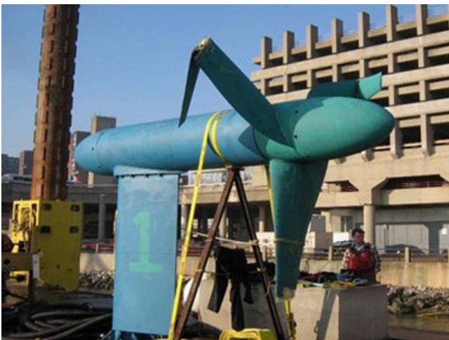
Fig. 1. Failed blade of a TCT.
