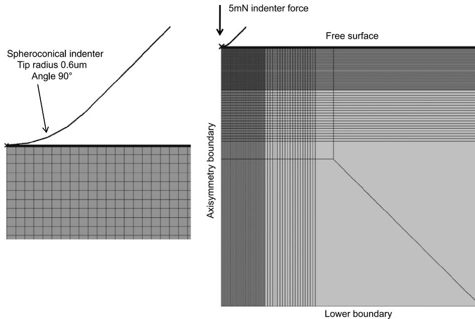
**Fig. 1 – Axisymmetric FE mesh showing boundary conditions and indenter force (right), close-up view of mesh in the vicinity of indenter tip (left).**
