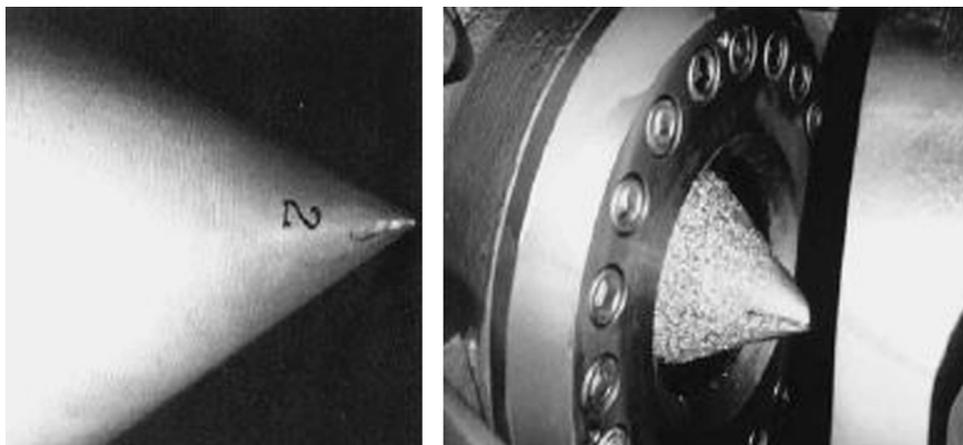
**Fig. 1.** A sample of synergetic erosion inside a Pelton turbine. (a) Initial stage with 300-hour operations with silt erosion on the needle tip; (b) subsequent synergetic erosion with 600-hour operations on the needle tip. The figure was adapted from Brekke et al. [24].
