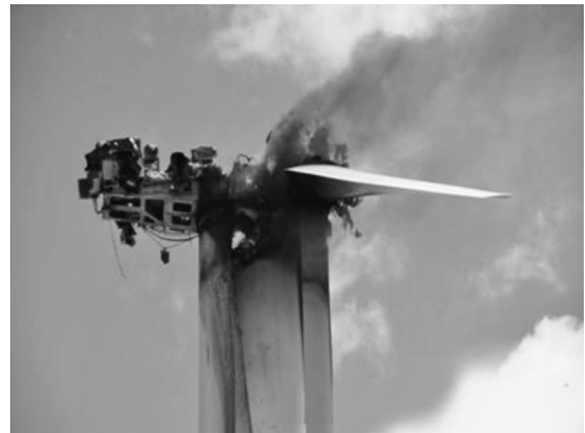
Fig. 1. 1.5 MW wind turbine nacelle fire in Xilingol wind farm in Inner Mongolia.
