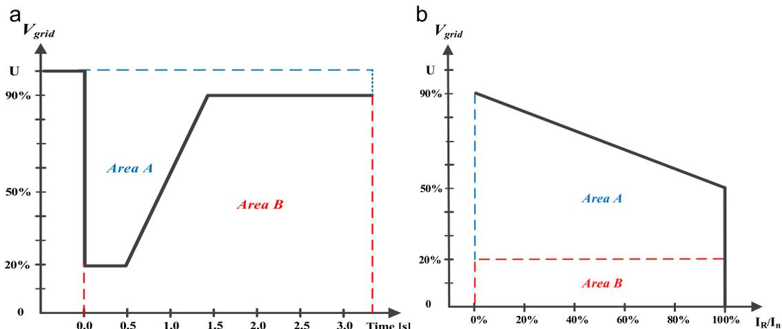
Fig. 1. Danish grid codes. (a) LVRT requirement. (b) Reactive power support requirement.
