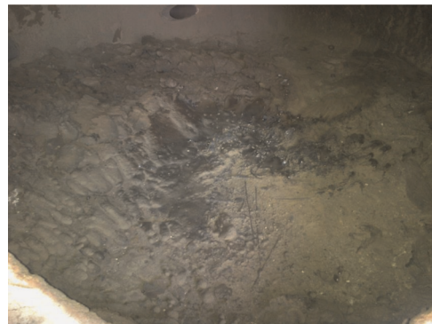
Fig. 2. Vitrified bottom ashes in a burner fuelled with sawdust.
