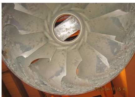
48 MW*3 Francis turbine at Kaligandaki Power plant, Nepal [5]
