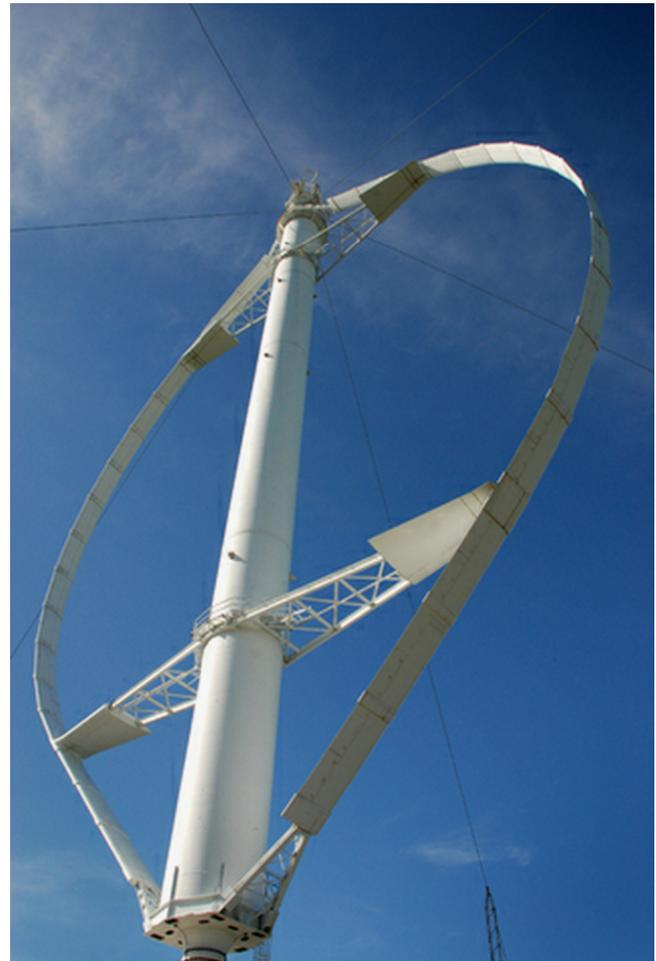
Fig. 1. 3.8 MW Éole VAWT  $\Phi$ -rotor.
