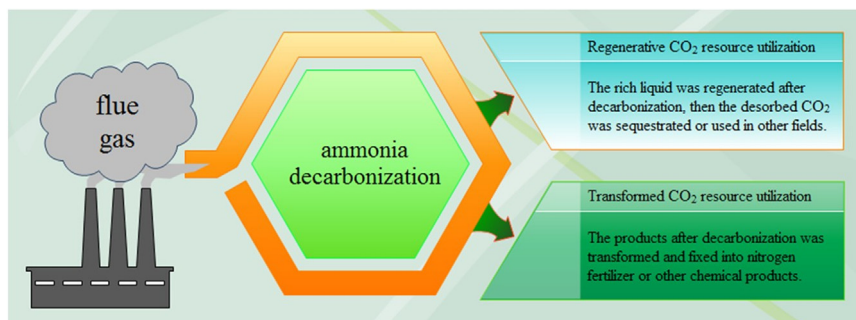
Fig. 1. Two feasible resource paths based CO 2 capture using ammonia solution in power plants.
