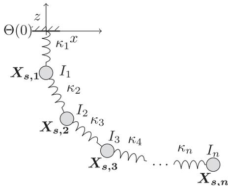
Fig. 1. Schematic view of the model of the drillstring. The drillstring is considered as a set of  $n$  blocks with masses and moment of inertias denoted by  $m_i$  and  $I_i$ , respectively. These blocks are connected to  $n$  springs with spring constants that are denoted with  $\kappa_i$ .
