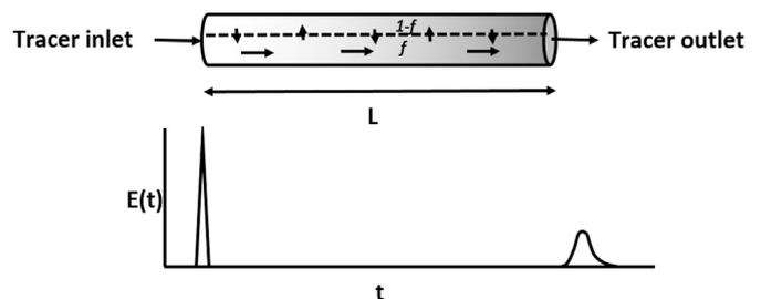
Fig. 1. Schematic of a pulse tracer test in a porous medium with a mobile fraction  $f$  and immobile fraction  $1 - f$ .
