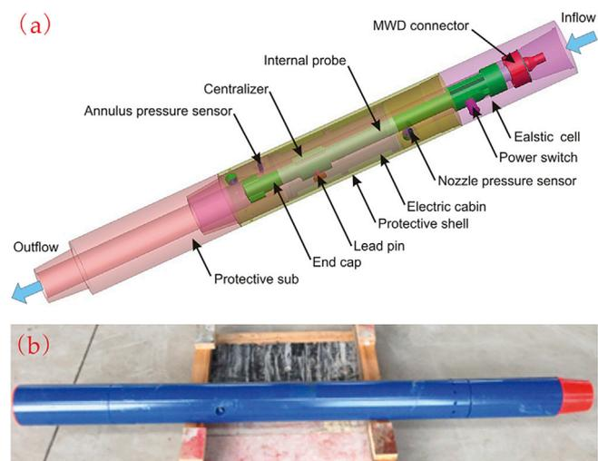
Fig. 2. The developed downhole monitoring apparatus. (a) Schematic diagram; (b) Picture of real products.
