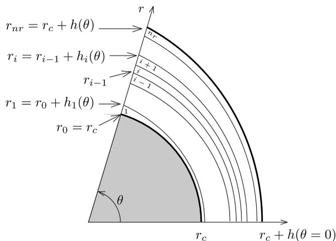
Fig. 2. Schematic of the annular domain decomposition into  $n_r$  layers for a given  $z$ .
