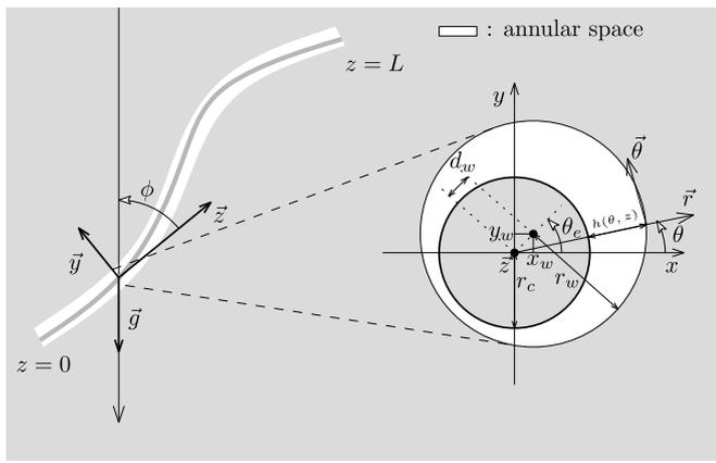
Fig. 1. Schematic of the annular space geometry and geometrical variables.
