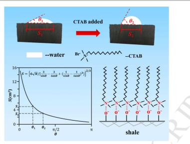
After adding CTAB to the WBM or water, CTA<sup>+</sup> is easy to adsorb on the surface of shale via an ionic bond (the red dotted line), forming a hydrophilic base toward the shale and a lipophilic base toward the WBM or water, thus, increasing the contact angle and decreasing the contact area with shale.
