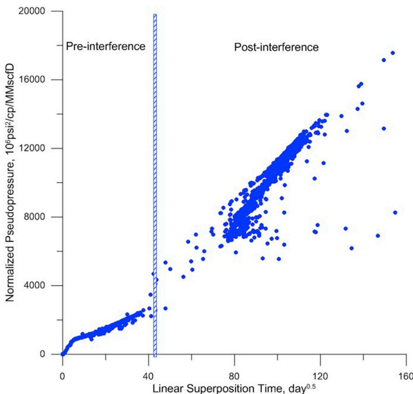
Fig. 2. Interference Linear Superposition Time plot.
