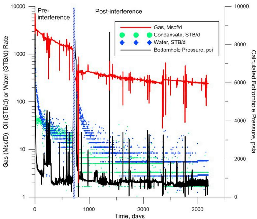
Fig. 1. Gas rate versus time pre- and post-interference.
