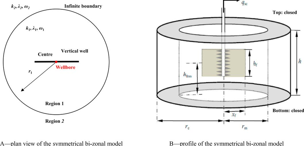
Fig. 1. Schematics of the plan view and profile of the symmetrical bi-zonal model for a partially penetrating fractured well (Zhao et al., 2015).
