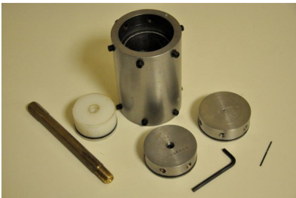
Fig. 2.1. Cell body, upper cap, modified lower cap, piston (white) and removal tool (yellow). (For interpretation of the references to color in this figure legend, the reader is referred to the web version of this article.)
