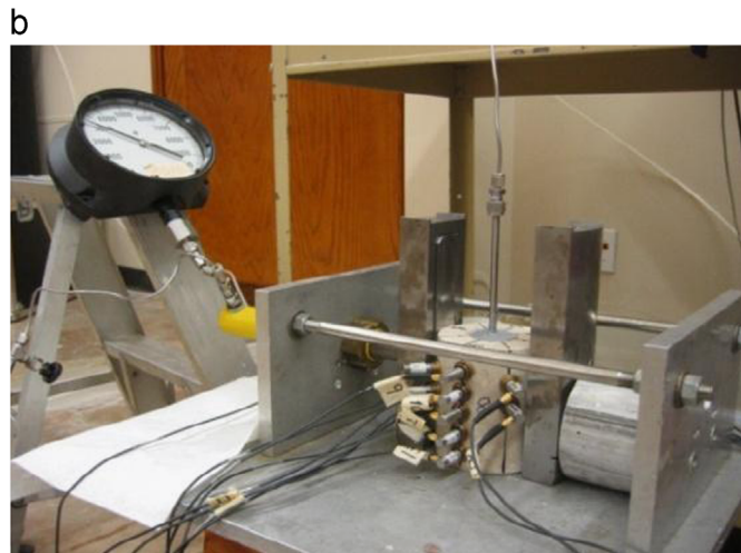
Fig. 1. (a) 3-D plan and side views of a 4-in. diameter sample completed with 0.12 in. ID mini-casing. Fluid ports in the mini-casing are located at the midpoint of the sample (black triangles). (b) Lyons sandstone is shown instrumented and stressed horizontally while undergoing hydraulic fracture stimulation. In the foreground, note the dense vertical subarray of sensors.
