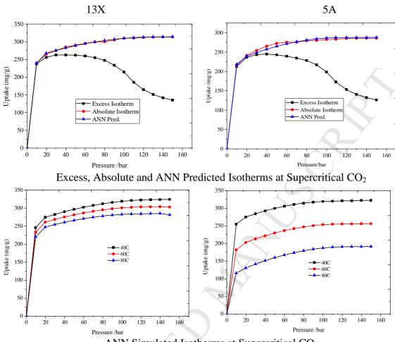
ANN Simulated Isotherms at Supercritical CO<sub>2</sub>
