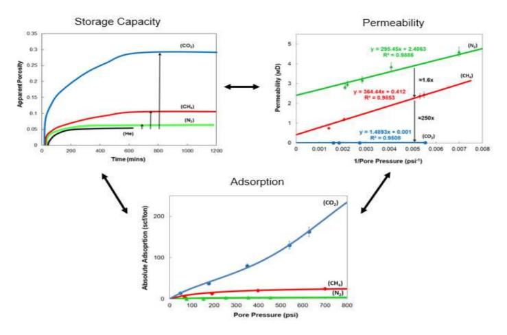
We present an apparatus for and simultaneous measurements of gas storage capacity, permeability, and adsorption of shale. The experimental observations were corroborated using a grand canonical Monte Carlo (GCMC) simulation.
