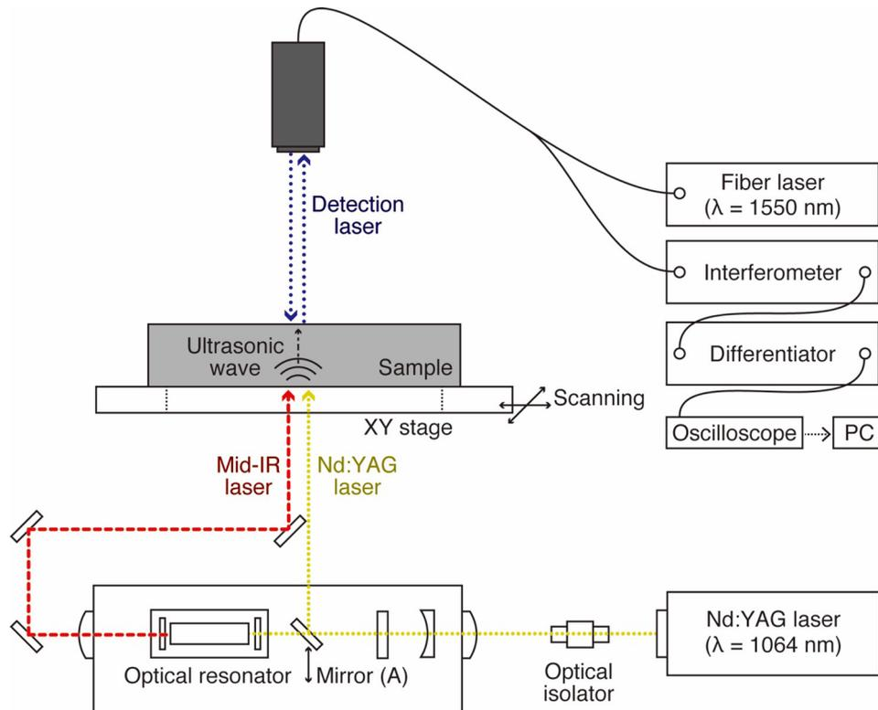
**Fig. 1.** The schematic diagram of the mid-IR laser ultrasonic testing system. The optical resonator converts the Nd:YAG laser to the mid-IR laser for the ultrasonic generation. The Nd:YAG laser was also used for the ultrasonic generation source by inserting the mirror (A).
