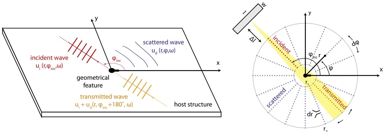
Fig. 1. Presentation of the incident, scattered and transmitted wave fields (left). Configuration for scattering characterization (right).
