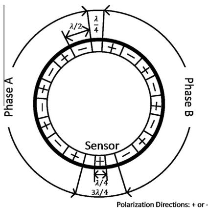
Fig. 1. Sketch of polarization directions of piezoelectric ceramics attached on stator.
