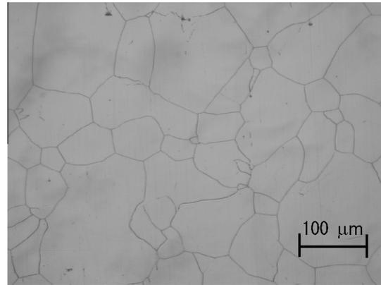
Fig. 2. Microstructure of the test specimen.
