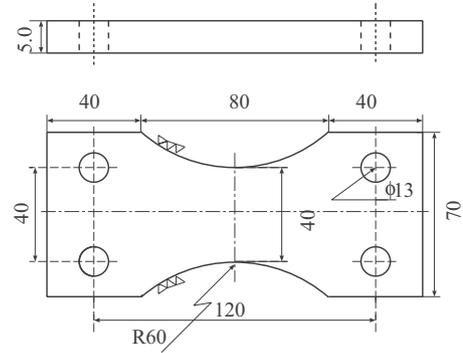
Fig. 1. Specimen configuration.
