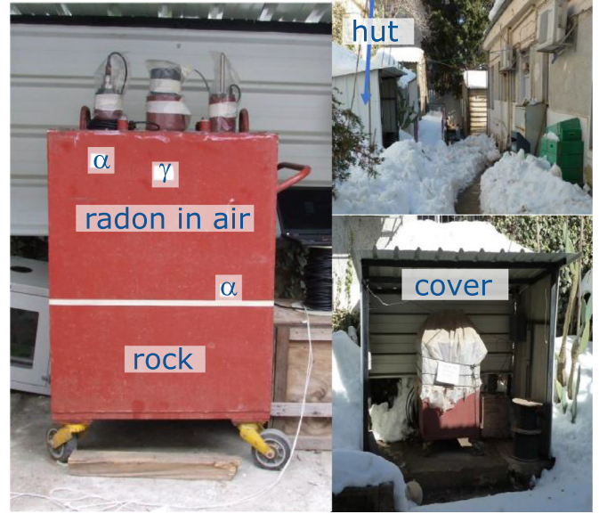
Fig. 2. Front view of the tank with sensors at GSI [11], with indications of the level of the phosphorite rock at the bottom and the positions of the gamma (middle) and two alpha sensors. The covering hut is open to the south, such that the instrument is partially exposed to rainfall driven by southern wind and to light from the Sun and the adjacent building. The external parts of the electronics are covered with large polyethylene sheets (see bottom right picture) for protection.
