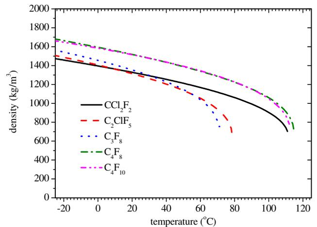
Fig. 1. Variation of liquid densities with temperature [19].
