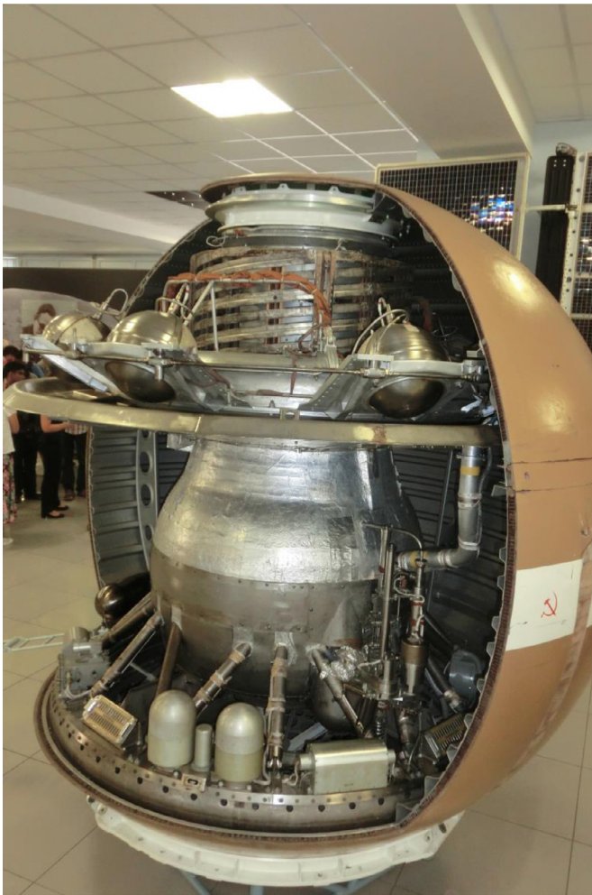
Fig. 1. VEGA lander and entry system on display in the Lavochkin museum in Moscow. (Photo: R. Lorenz – high-quality version of this image and others are included in the /extras directory of the PDS archive). Note the spherical entry vehicle, the silvered spherical lander attached to its landing ring on which various instrumentation is mounted: surface sampling mechanism is at right. At top above the braking disk to provide stable drag in descent are spherical helium tanks to inflate the balloon.
