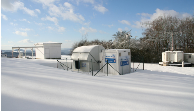
Fig. 1. Projectsoft BlueEye600 robotic observatory located in Ondřejov, Czech Republic. The alt-azimuth telescope is of Ritchey–Chrétien type with the primary diameter d = 600 mm.
