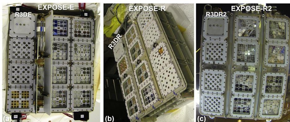
Fig. 1. a/b/c. External view of the R3D instruments (in the upper left corner of the pictures) as mounted on the ESA EXPOSE facilities. (The EXPOSE-R2 picture (Fig. 1c) was taken by the Russian cosmonauts G. Pedalka and M. Kornienko on August 15, 2015 during an examination of the facility outside the Russian “Zvezda” module.) (Picture credit ESA/RKA).
