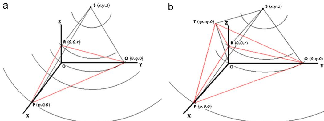
Fig. 1. (a) Geometry of positions of microphones and the thunder source for three microphone system. (b) Geometry of locations of microphones and thunder source for the model with four microphones.
