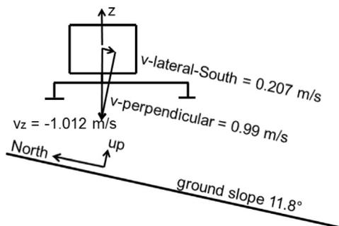
Fig. 1. Incoming velocity vector and its components in perpendicular and lateral direction in East view. The outgoing velocity is in South-East direction (more details Fig. 3).
