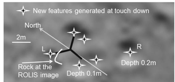
Fig. 4. Superposition of the ROLIS “rock” and the OSIRIS (Credit: ESA/Rosetta/MPS for OSIRIS Team MPS/UPD/LAM/IAA/SSO/INTA/UPM/DASP/IDA) image. New features produced by the lander touch-down at the Agilkia site are marked by star symbols. Note: The alignment accuracy between ROLIS and OSIRIS images is about 0.4 m. The new feature most left is marked L, the most right one R.
