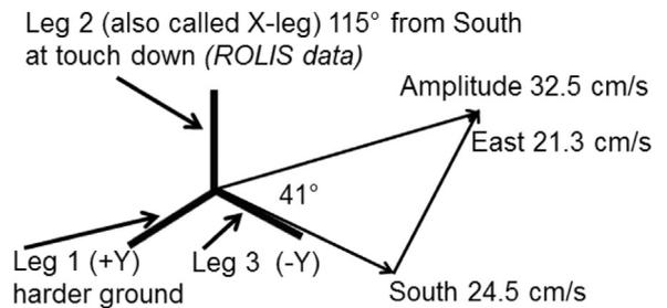
Fig. 3. Lander velocity vectors, sketched in the lander reference system. The inbound velocity is perpendicular to the plane of the drawing. The outbound velocity in the lander coordinate system is almost in the paper plane (like indicated), since the  $v_z$  velocity is only 2 cm/s. The direction of the velocity vector was changed by almost 90° at touch-down. East and South are slightly tilted to the paper plain.
