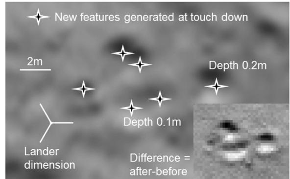
Fig. 2. OSIRIS (Credit: ESA/Rosetta/MPS for OSIRIS Team MPS/UPD/LAM/IAA/SSO/INTA/UPM/DASP/IDA) difference image of the touch-down area – exposure after minus exposure before touch-down. New features for the lander ground contact spread over about 10 m, while the lander footprint area has 3 m diameter only. The lander legs dimension is sketched for comparison. The pattern in the surface shows that just a reflection on the surface cannot explain these features.
