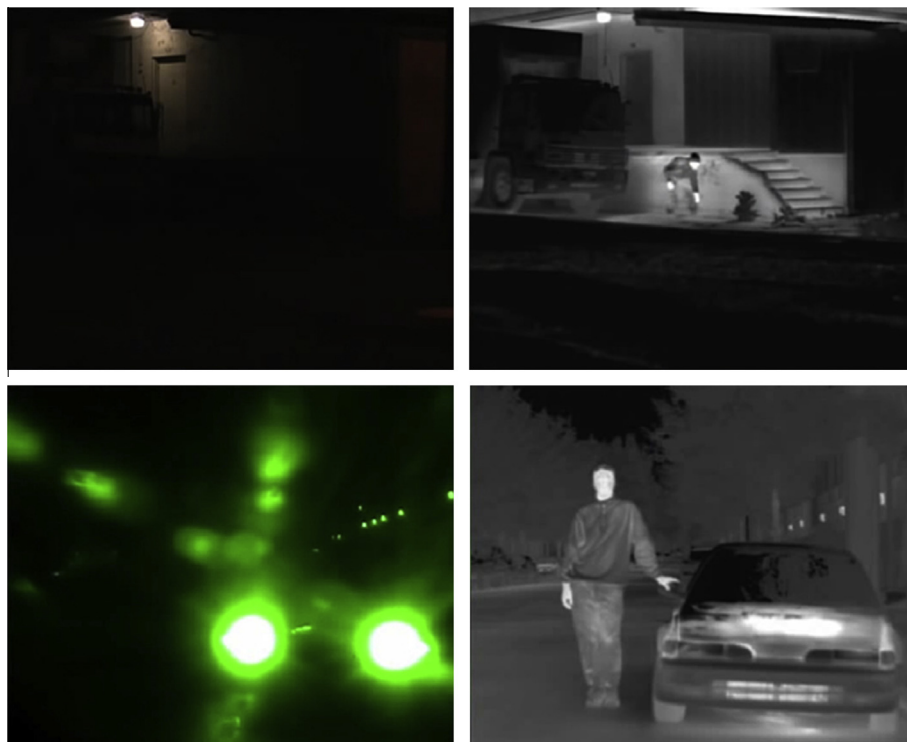
Fig. 1. Human being is not perceptible in the visible image on the left column, but can be detected from thermal images on the right (image courtesy of Infiniti Optics: http://www.infinitioptics.ca ).
