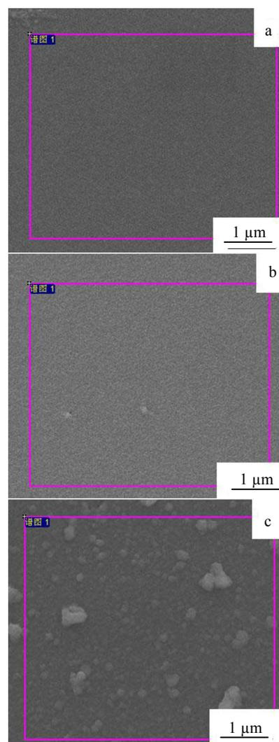
Fig.2 SEM images of surface morphologies of the thin films as-deposited (a) and thermally annealed at 473 K (b) and 623 K (c)
