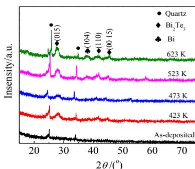
Fig.1 XRD patterns of co-sputtered Bi<sub>2</sub>T<sub>3</sub> thin films as deposited and those after annealing at different temperatures
