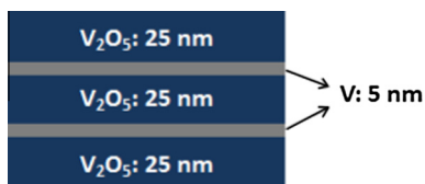
Fig. 1. Schematic diagram of the multilayer sandwich structure.
