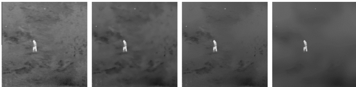
Fig. 1. Smoothing result with different \sigma_s and \sigma_v for Gaussian function. (a) Original image, (b) smoothing result with \sigma_s = 3 and \sigma_v = 0.05 , (c) smoothing result with \sigma_s = 12 and \sigma_v = 0.05 , (d) smoothing result with \sigma_s = 12 and \sigma_v = 0.15 .
