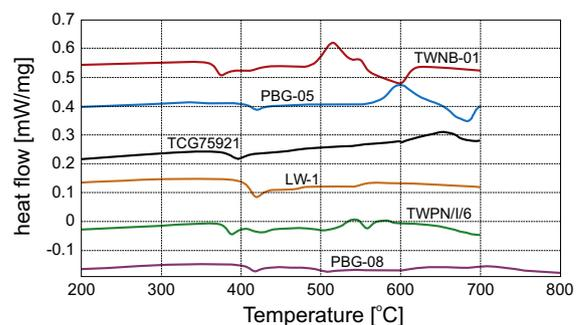
Fig. 2. Curves of differential scanning calorimetry of the considered glasses.
