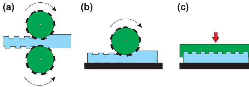
Fig. 1. Basic types of the hot embossing process.
