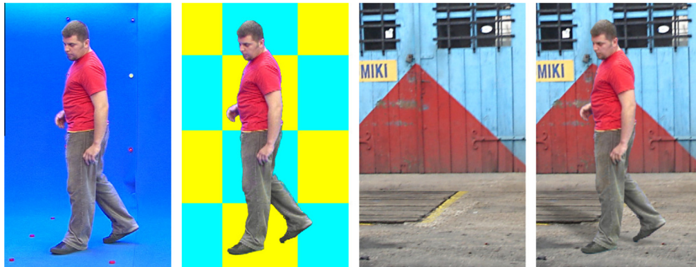
Fig. 2. Example of applications. From left: Original image with markers; actor after keying; CG scenery; final composite [6].
