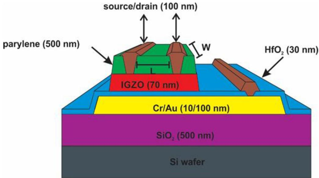
Fig. 1. Schematic of the bottom gate top contact IGZO TFT structure fabricated for this study.
