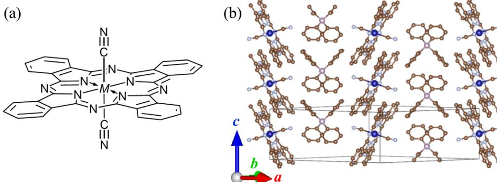
Fig. 1. (a) Molecular structure of  $M(\text{Pc})(\text{CN})_2$ . The  $M$  indicates the transition-metal atom. (b) Crystal structure of  $\text{TPP}[M(\text{Pc})(\text{CN})_2]_2$  [9–11].
