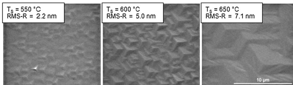
**Fig. 2.** SEM images of GaAs layers grown at different substrate temperatures 550 °C, 600 °C and 650 °C with corresponding rms-roughnesses 2.2 nm, 5.0 nm and 7.1 nm. As:Ga BEP is set to 116.6 and cracker temperature to 500 °C.
