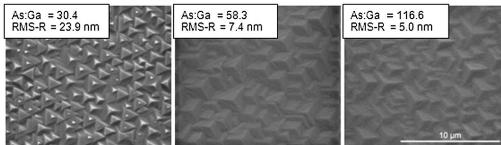
**Fig. 1.** SEM images of GaAs layers grown with different As:Ga BEP ratios 30.4, 58.3 and 116.6 (corresponding to growth rates of 0.72 μm/h, 0.36 μm/h and 0.18 μm/h) with rms-roughnesses 23.9 nm, 7.4 nm and 5.0 nm. Substrate temperature is set to 600 °C and cracker temperature to 500 °C.
