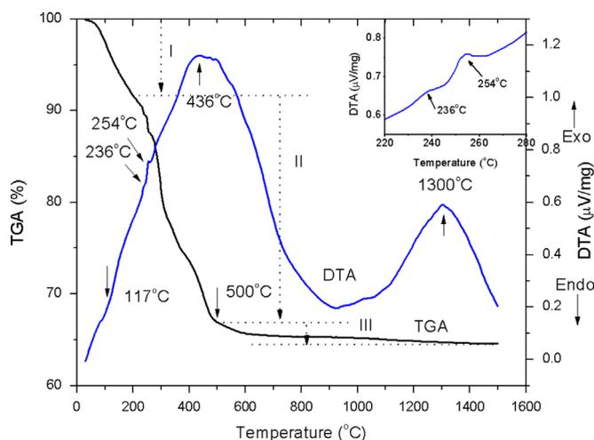
Fig. 1. TG-DTA curve of dry gel of SGL sample.
