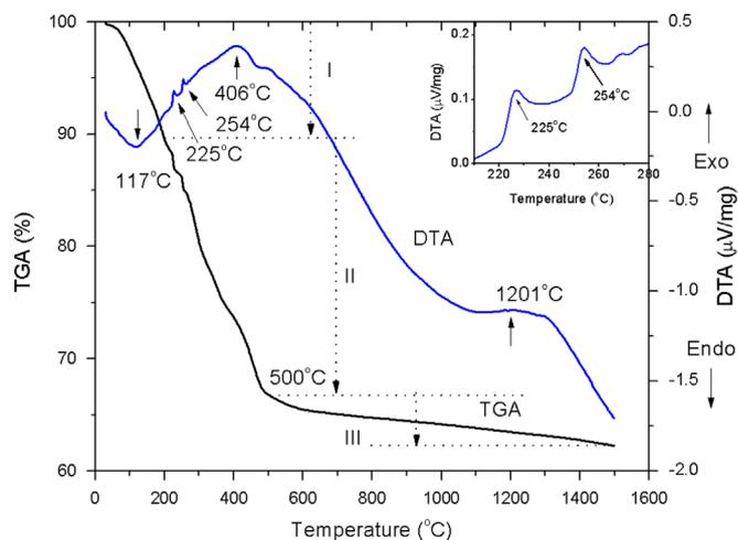
Fig. 2. TG-DTA curve of dry gel of SGLS Sample.
