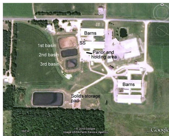
Fig. 1. Configuration of the WI dairy. Manure in the measured basins (1 and 2) came from barns 1 and 2 and the parlor and holding area illustrated in a GoogleEarth® image. Solids are separated at the separator and liquids pumped to inlet on the east side of the 1st basin.
