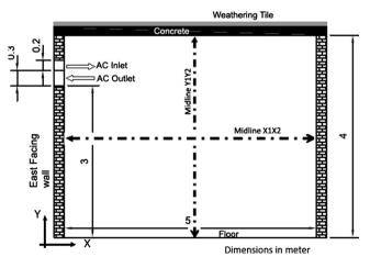
Figure 1 Computational model of test case room.
