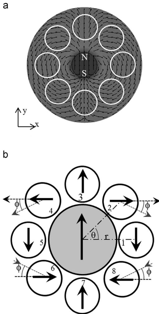
**Fig. 1.** (a) Schematic showing the concept of automatically aligning eight magnets into a Halbach orientation. Polarization direction of the magnetic field obtained from a diametrically magnetized cylinder located at the center of the figure is denoted by the arrows. The locations of the eight magnets to be aligned by the center magnet are denoted by white circles. (b) Schematic showing a model for the automatic alignment.
